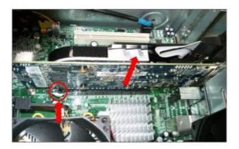
3.4 Disconnect 6 PIN power cable in USB 3.0 Card(option)
